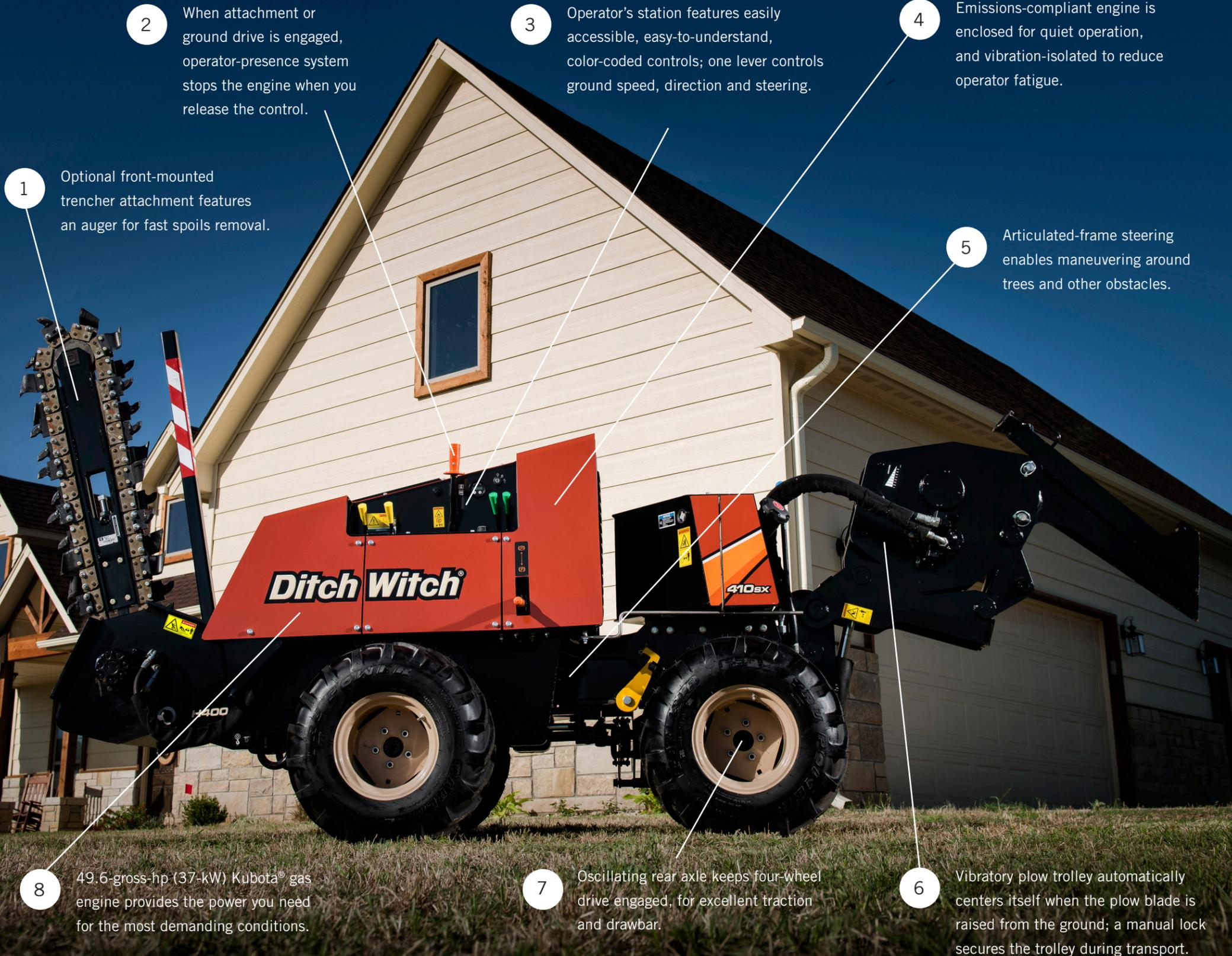
1 Optional front-mounted trencher attachment features an auger for fast spoils removal.
