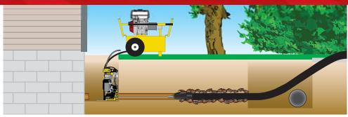
A typical job site with the PortaBurst® Lightning set up at the house. Alternatively the unit can be set up in the basement or at the clean out. The burst head is pulled through the lateral, bursting the existing pipe, while simultaneously pulling in the new pipe.
