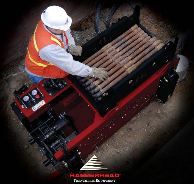
PRODUCTIVE, COMPACT 100 TON STATIC PIPE BURSTING SYSTEM HYDROBURST® HB100
