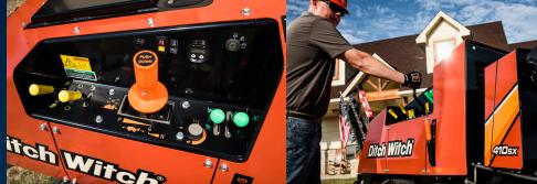
The Ditch Witch® 410SX is the most outstanding articulated-steer vibratory drop plow in its horsepower class. With dozens of innovative features, including an oscillating rear axle that keeps the machine's fourwheel drive engaged, the 410SX quickly and efficiently installs communication lines, natural gas and water services, or a complete underground sprinkler system without digging a trench. Need a trench? The 410SX can do that, too.
