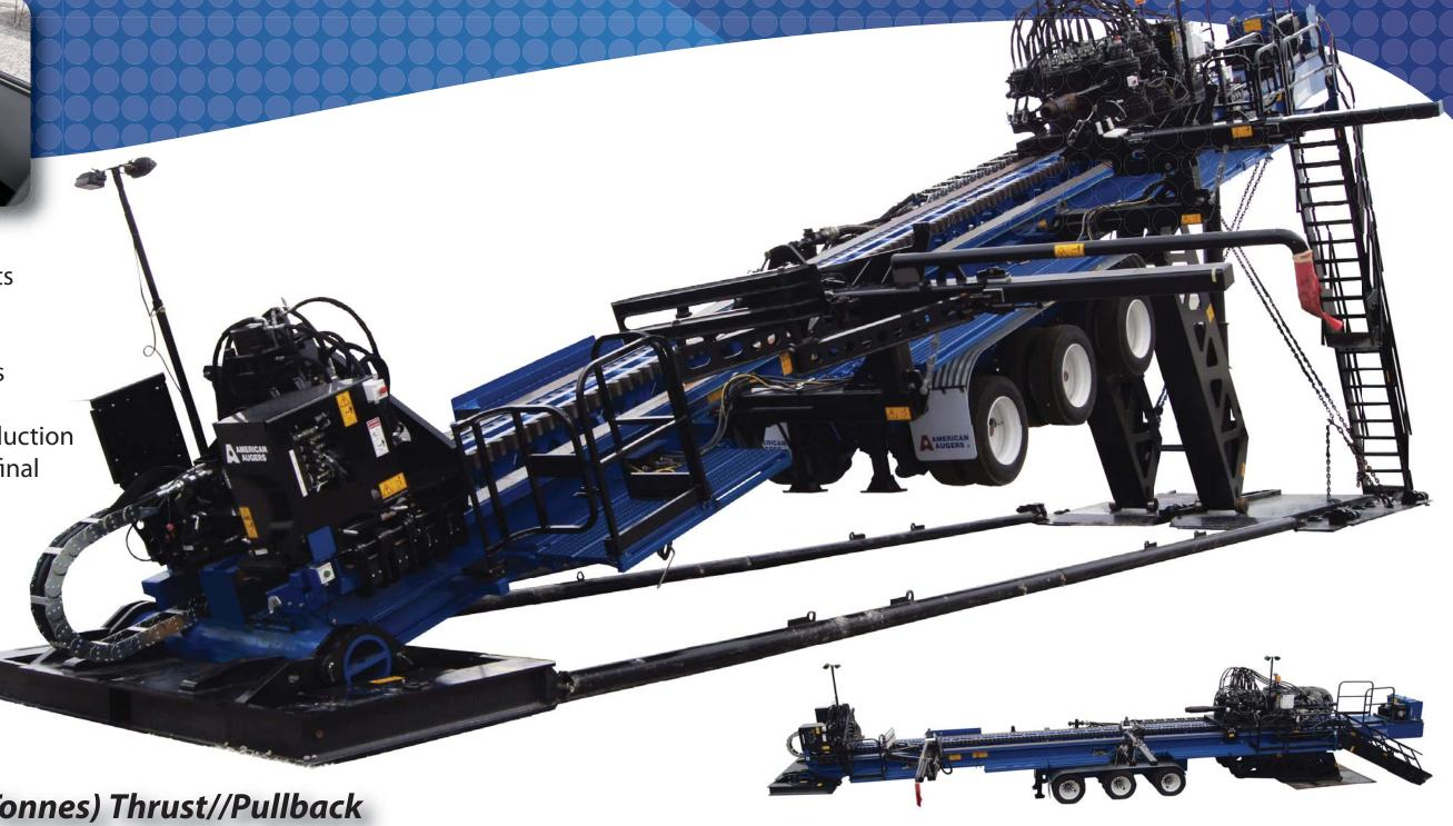
660,000 lbs. (300 Tonnes) Thrust//Pullback
